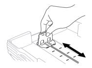
3 Fan the paper well. Load paper in the paper cassette. Press down on the paper to flatten it in all four corners, keeping the paper level below the guide. The cassette can hold up to 250 sheets of 20 lb (75g/m<sup>2</sup>) paper.
